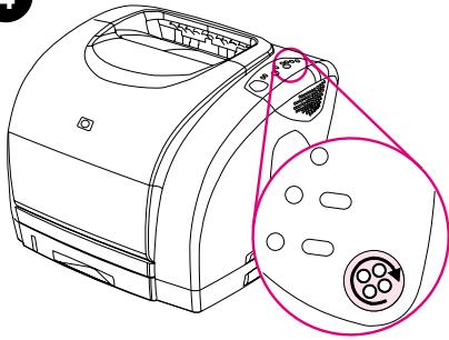
If the print cartridge that you want to replace is not in the access position, close the top cover and press **ROTATE CAROUSEL**. Repeat until the print cartridge is in the access position.
