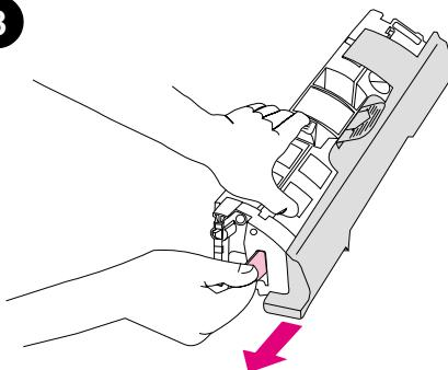
Place the new print cartridge on a flat surface. Pull the orange tab straight out to remove the sealing tape.
