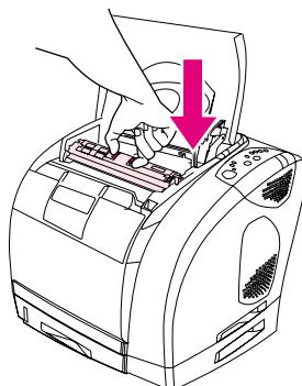
Hold the print cartridge by the blue release levers and lower the cartridge straight down into the carousel until it is firmly in place.
