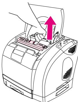
Squeeze the blue release levers and remove the used print cartridge from the printer.
