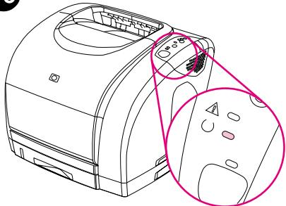
The light on the control panel that corresponds to the print cartridge you replaced should be off. The green Ready light should be on.
