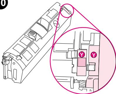
Make sure the color label on the right side of the print cartridge matches the corresponding slot in the printer.
