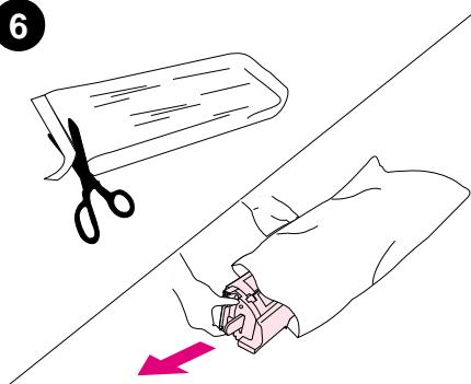
Remove the new print cartridge from the bag. Place the used print cartridge in the bag for recycling.
